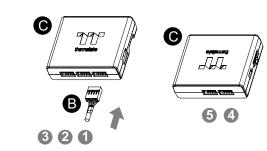
Connect the fan cable onto the controller.
