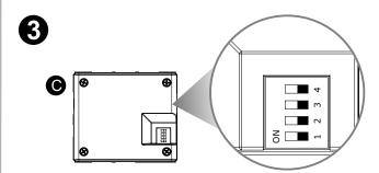
Set the DIP switch on the back side of the controller to assign the number of the controller
