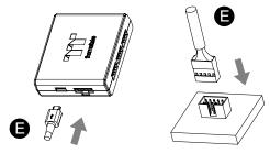
Connect the controller cable onto the mainboard (USB 2.0 9 pin) and controller.
