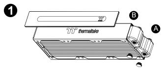
Install the LED Module on the radiator.
